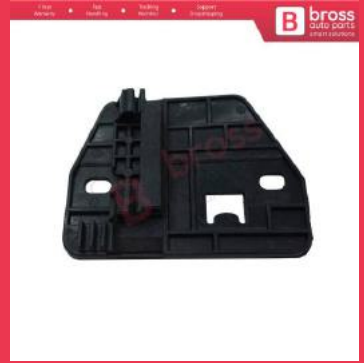
BWR1181 Renault Master MK2 Mascott Opel Movano A Iveco Daily 3 4 Nissan Interstar X70 7700352494 İçin Ön Sol Kapı Cam Kriko Tamir Klipsi
